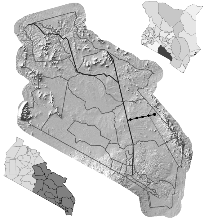
Figure 7. A pipeline spur extends northwest in Imbirikani Group Ranch to Chyulu Hills, from the Nolturesh Pipeline, which flows north. The pipelines are shown in heavy lines. A water source at the end of the spur was modeled (large symbol), and sources every 5 km along the spur were modeled (smaller symbols). Topography is shown in shades of grey, and insets show the location of the study area in Imbirikani Group Ranch, and the ranch in Kenya.
